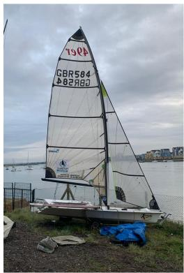
The rudder and dagger board are made out of fibreglass which we had to restore with gel coat because they were old and very worn. The spinnaker pole is made out of carbon composite allowing it to bend under extreme tensions and not just snap, along with the end cap to prevent breaking.
